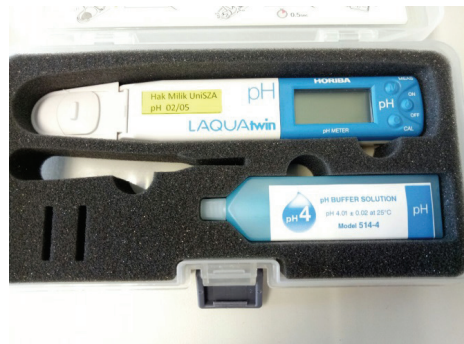
Fig. 1. Rheometer to measure the viscosity. Fig. 2. Compact pH-meter for pH measurement.
